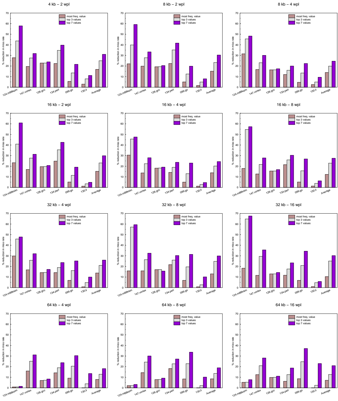
Figure 12: % reduction in miss rates: DMC vs DMC + FVC (top 1 vs 3 vs 7 frequent values).
