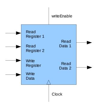
A register file can be implemented with a multiplexer for each read port, a decoder for the write port and an array of registers built from D flip-flops.
