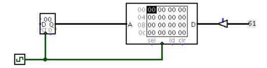
Build a circuit in *Logisim* that writes the value 0x61 to every memory location. Your circuit should allow the user to reset the counter anytime. In addition, the circuit should stop writing values to memory after it has already written all memory locations.
