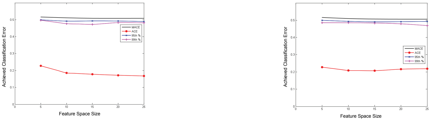
Figure B4: PACE analysis using a SVM-based classifier using the simple separability scoring criterion, with a 0.6 MAC threshold. Left Panel: performance without peak selection. Right panel: performance with peak selection.
