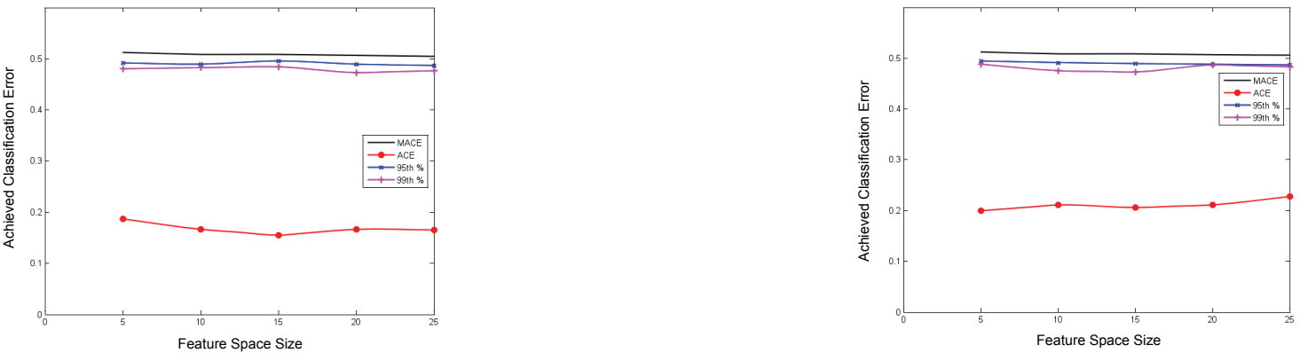
Figure B6: PACE analysis using a SVM-based classifier using the weighted separability scoring criterion, with a 0.6 MAC threshold. Left Panel: performance without peak selection. Right panel: performance with peak selection.
