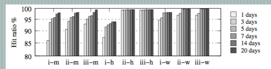
Figure 2: Overlap in daily working sets for the mail (m), homes (h), and web-vm (w) workloads. (i) Reads and writes against working set, (ii) Reads against working set and (iii) Reads against working set, recently offloaded writes, and recent missed reads.
