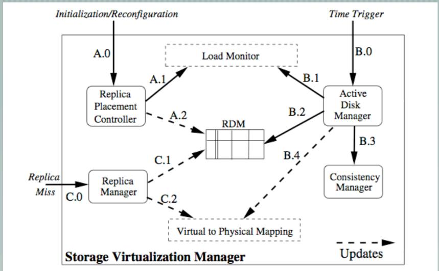
Figure 4: **SRCMap integrated into a Storage Virtualization Manager.** Arrows depict control flow. Dashed/solid boxes denote existing/new components.
