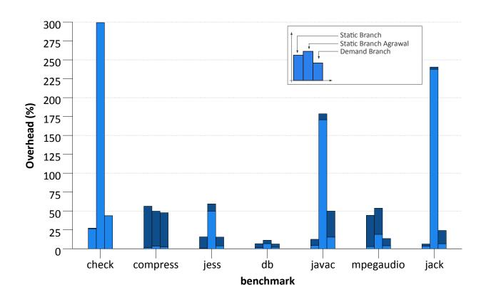
Figure 4.10: Branch planning overhead (light blue) and instrumentation (dark blue).
