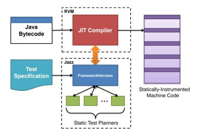
Figure 3.3: Static instrumentation in Jazz.
