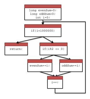
Figure 1.1: Static instrumentation is not removed after recording coverage.
