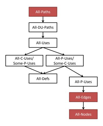
Figure 2.1: Partial subsumption hierarchy for adequacy criteria.
