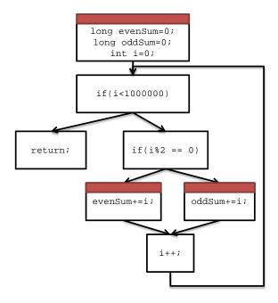
Figure 1.2: Agrawal's algorithm statically places fewer instrumentation probes.
