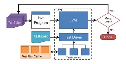
Figure 6.2: Cached test plans can be reused across the test cases in a suite.
