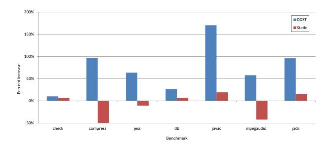
Figure 5.3: Change in branch misprediction rate for DDST and Static.
