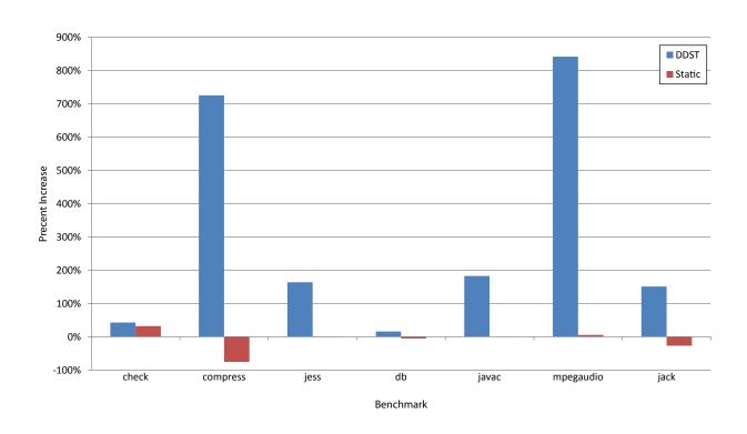
Figure 5.4: Change in DTLB miss rate for DDST and Static.
