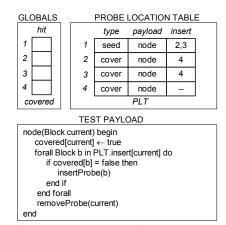
Figure 4: Example test plan for node coverage
