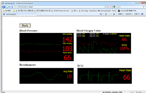
(b). The remote monitoring screen of the detailed physiological data on the web browser
