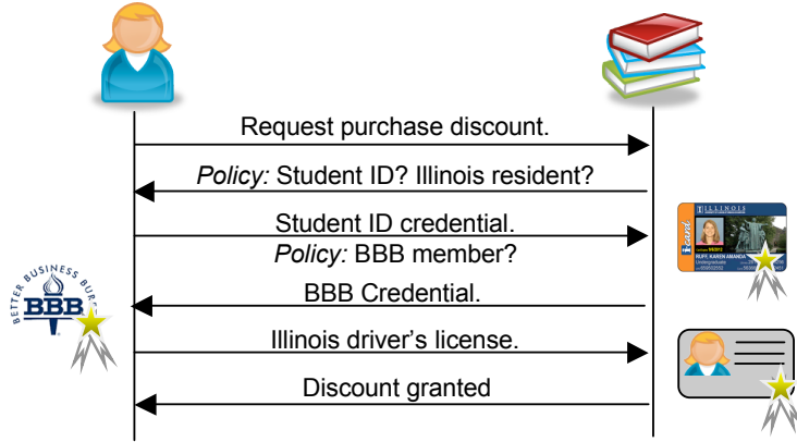
Figure 1.2: A trust negotiation session in which a user negotiates for a student discount at a bookstore.
