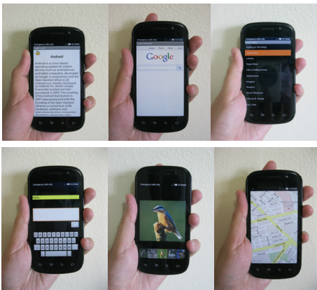
Figure 9. Sample LensGesture applications. From left to right, top to bottom - LensLock, LensCapture, LensMenu, LensQWERTY, LensAlbum, and LensMap.
