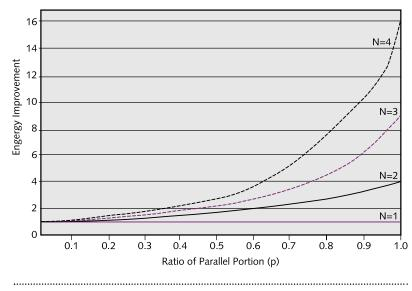
Figure 1. Achievable dynamic energy improvement assuming  $\alpha = 3$  and using 1, 2, 3, and 4 processors, given the ratio of serial and parallel work in a program.
