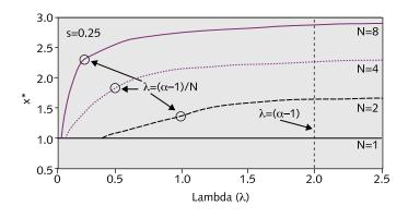
Figure 4.  $\lambda$  changes  $x^*$ , the speedup of a program when its energy consumption is minimized.  $x^*$  saturates at the maximum speedup that Amdahl's law dictates when  $\lambda > \alpha - 1$ . We assume that  $\alpha = 3$ .
