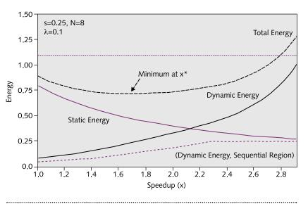
**Figure 6.** Optimal energy, given the speedup of x, with  $\alpha = 3$ . Total energy is the sum of dynamic and static energy. This plot also shows dynamic energy for the sequential region. The thick dotted line shows the sequential machine's energy consumption. Given these parameters, the maximum speedup (Amdahl's law) is 2.909, and  $x^* = 1.684$ , according to equation (14). The dynamic energy of the sequential region saturates at 2.286, according to equation (21).
