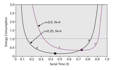
Figure 3. Dynamic energy consumption vs. t (serial time) for two cases, s = 0.25 and s = 0.5 when N = 4. The bound of t is marked with X (when  $f_s = F_{max} = 1$ ) and O (when  $f_p = F_{max} = 1$ ). The minimum energy point in each curve (at  $t = t^*$ ) is marked with a filled rectangle.
