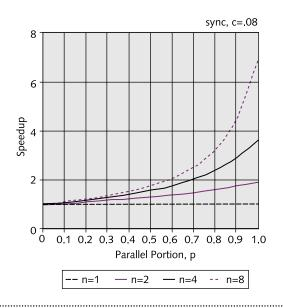
Figure 7. Achievable dynamic energy improvement, after accounting for a synchronization overhead of  $0.08 \log n$ . As in Figure 1,  $\alpha = 3$ .
